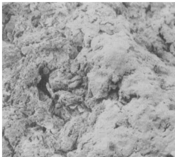
Figure 1. Scanning electron micrograph of the magnesium oxide granules. Particle size: 0.1–0.16 mm. Magnification: 2000 \times .
